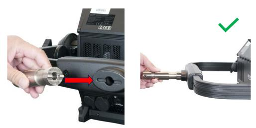
2. Locate the notched face of the junior pin, and hold it against the clamp mounting point located on the top side of the yoke. The notched surface of the junior pin must sit flush against the matching groove on the surface of the clamp mounting point.
