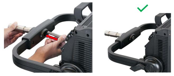
3. Thread the junior pin bolt in through the under side of the mounting yoke, making sure that the bolt engages the threaded hole in the junior pin. Tighten securely with a 10mm hex key. The junior pin is now ready for attachment to a clamp or stand.
