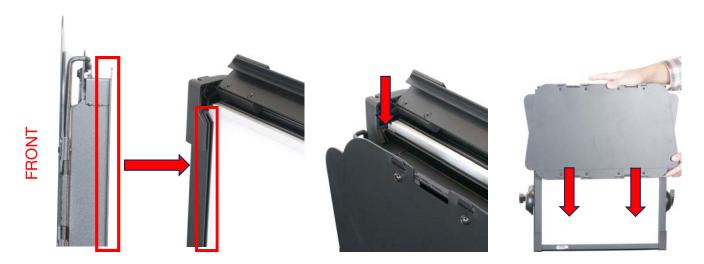
2. The inner frame of the fixture contains an empty mounting slot located just in front of the removable diffuser. Align the mounting rail on the rear of the barn door with this empty mounting slot, and slowly lower the barn door into place.
